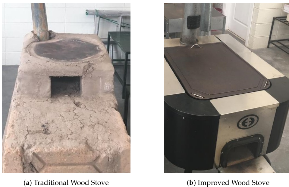
Figure 3. Traditional-style stove commonly used in Honduras, in comparison with the Improved cookstove model (Ecofogon) being distributed by the Honduran government. Pictures taken by author N.V.B. at the Improved Cookstove Evaluation Center (CEEM) at the University of Zamorano, Honduras.
