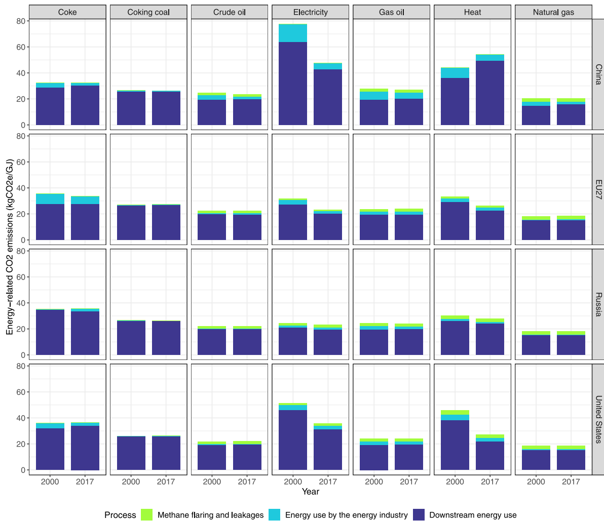
Fig. 7. Energy-related CO 2 e emissions for a unit of energy product delivered, disaggregated in terms of (i) emissions due to energy use by the energy industry, (ii) emissions due to downstream energy use by final demand sectors, and (iii) fugitive emissions due to methane flaring and leakages. Unit: kgCO 2 equivalent per GJ.
