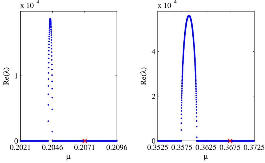
FIG. 2. (color online) Plots of the absolute value of the real part of the spectrum for various values of  $\mu$  for a wave with approximate amplitude  $2.3 \times 10^{-2}$ . The plot on the left is for  $\mu$  values near the zero/pole collision point  $\mu \sim 0.207$ , and the plot on the right is for  $\mu$  values near the zero/pole collision point  $\mu \sim 0.368$ . The  $\mu$  value for which the collision occurs is marked by a (red) cross.
